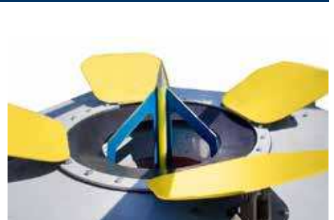
CUTTING KIT 3-blade configuration enhancing cutting performance
